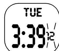
Repeatedly press MODE until TIME then the date and time appear. Then hold down SET/LIGHT/STP/RST. for about 3 seconds. The seconds digits flash.
